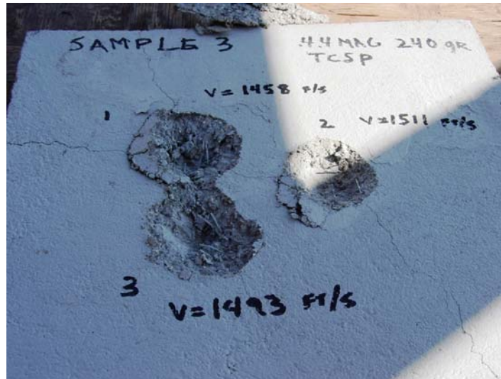
An IID fire wall panel stops a 44 Magnum bullet.
